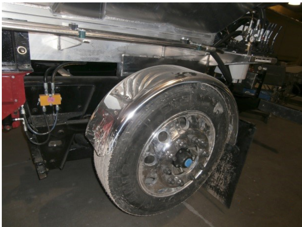
Figure 2-6. Support Spacer on an Aluminum Body
