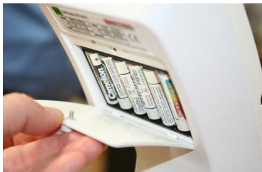
Figure 2-4. Batteries in Battery Chamber
