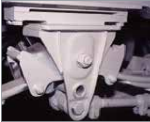
Equalizing suspension center hanger load cells
