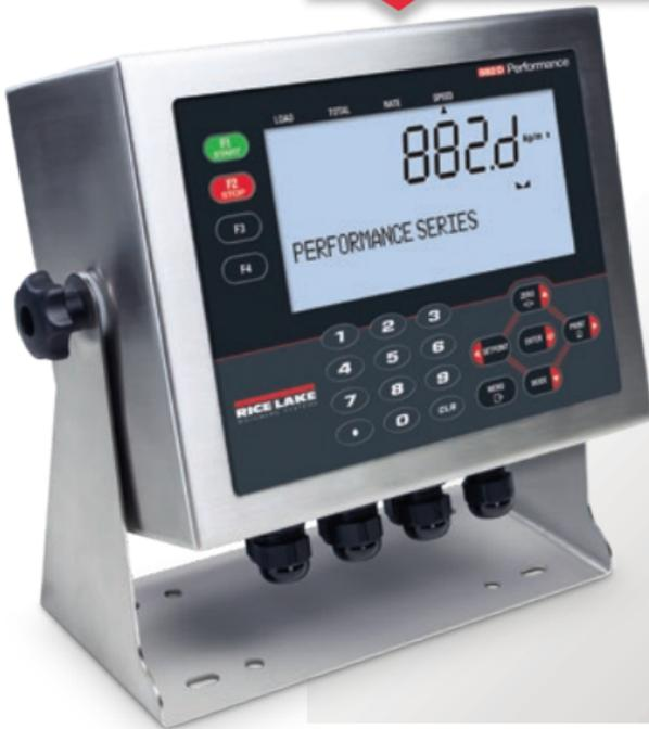
The 882D is specifically designed for belt scales. With advanced programming capabilities and an I/O option, the 882D can be customized to control product dosing or manage metering. A backlit LCD display makes viewing rate, speed and time convenient in almost any lighting condition. The 882D is also protected from weather with an IP66 stainless steel enclosure.
