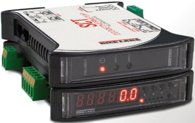
The SCT-2200 signal conditioning transmitter offers weight data control for PLCs without the space requirement of a traditional weight indicator. The SCT-2200 converts a scale's load cell signals to analog output, serial output or a specific network protocol.
