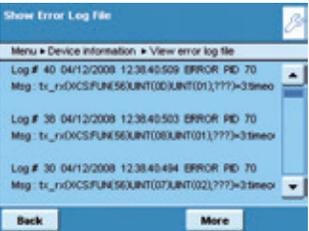
Logs important changes to the balance, so any errors or other non-conforming items can be quickly traced to the source.
