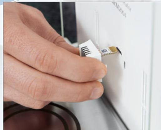
The climate sensors for temperature, humidity and air pressure are integrated in a small, compact, lightweight inter-changeable unit. They can be easily removed for DAkkS calibration.
