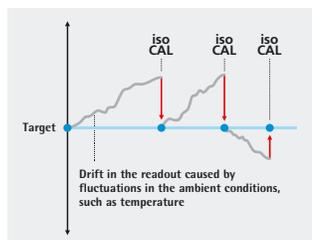
You can choose to have the isoCAL function perform fully automatic calibration and adjustment after a factory preset or user-definable interval has elapsed. In addition, when a factory preset or user-definable temperature difference is exceeded, isoCAL will automatically trigger calibration and adjustment again.
