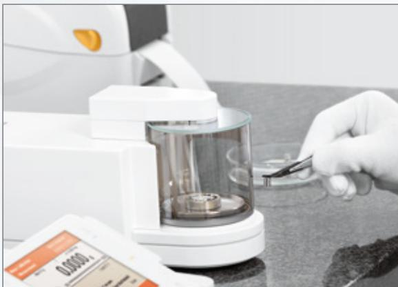
Cubis<sup>®</sup> MCM mass comparators deliver a full range of solutions for mass comparison by providing built-in climate sensors for temperature, humidity and air pressure, as well as user-guided workflows and readings of the results along with the measurement uncertainties.
