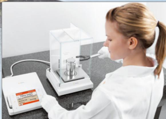
All Cubis® MCM mass comparators feature a separate display and control unit with an electronics unit isolated from the weigh cell to reduce the effects of heat generated by the electronics and of the warmth of the operator's hands.
