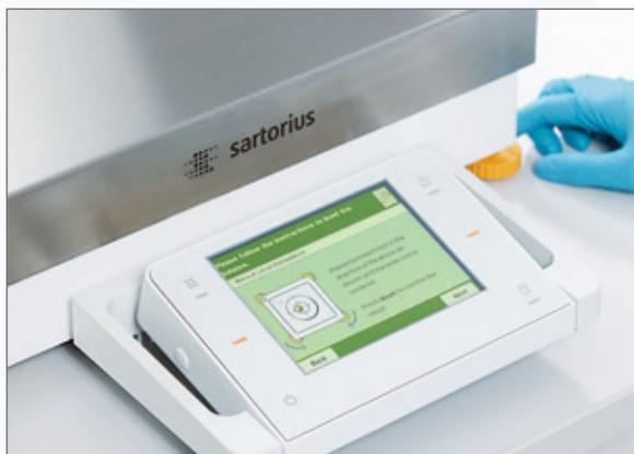
Cubis® continuously monitors whether it is perfectly level. Quick manual leveling takes just a few steps with interactive operator guidance prompts shown on the display.
